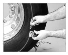
At the inner sidewall, connect the inner end fastener (the "split" in the outside cable can be opened to provide more space for connection the inside fastener.
