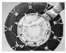
Install the rubber tensioner, always stretching the tensioner from one hook to the one farthest from it (use the included lever tool to make this installation easier.)
