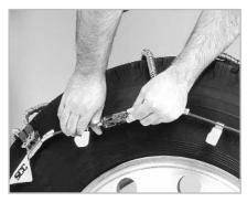
At the top of the outside cable, take the bushing end of the outside split side cable and thread it through the keyhole fastener. Grasp the outside cable with both hands and pull it toward you to create as much slack as possible. The connect the bottom fastener. See drawing below.
