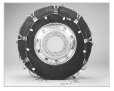
Park vehicle on firm level ground, away from traffic and turn off the engine. Set the emergency brake. Drape chain over the tire. Make sure that the smooth side of the crossmember hooks is against the tire sidewall. The tightener hooks on the side cable must be on the outside of the tire (towards you).
