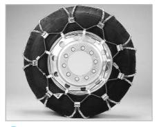
Use at least two rubber tensioners per chain and make sure that the tensioners are seated in all hooks. The vehicle may be driven with no further adjustment
